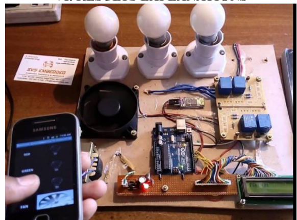
Figure 2. Hardware Prototype of the Android and Voice-Based Home Automation System
